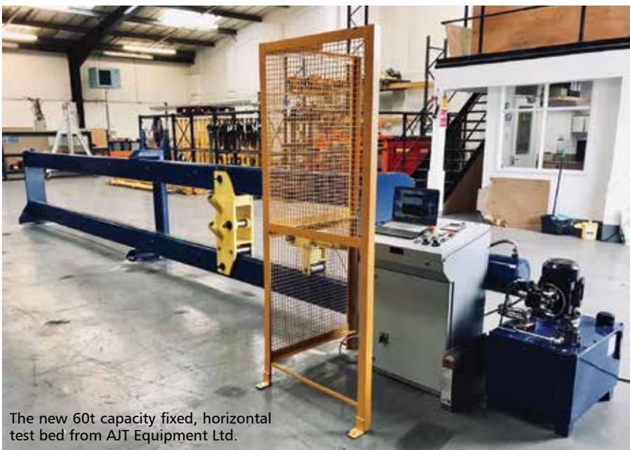
The new 60t capacity fixed, horizontal test bed from AJT Equipment Ltd.
