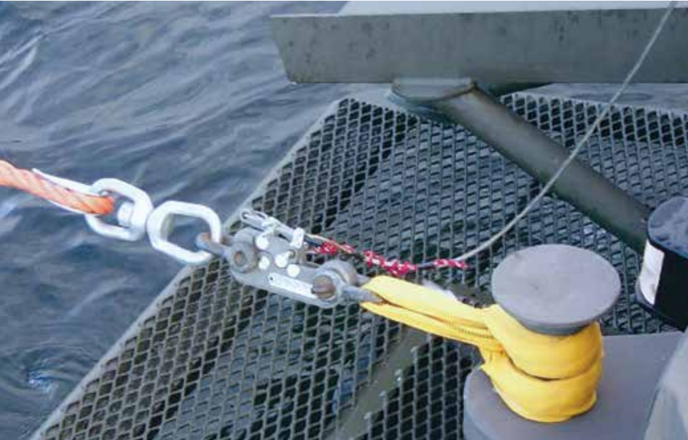
Sea Catch TR7 being tested for Swedish Navy's rescue and tow operations. Hitch pin in safety position, attached to the release lanyard enabling removal remotely.
