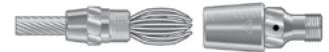
SLEEVE, PLUG & SOCKET: Plug driven in and strands closed to apply socket.
