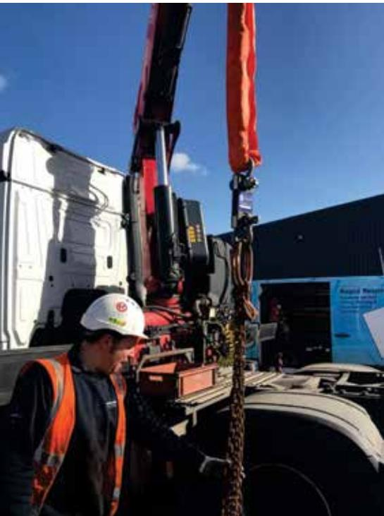
RRS used the load cell beneath the hook of a 34t capacity truck-mounted Fassi F365A crane.
