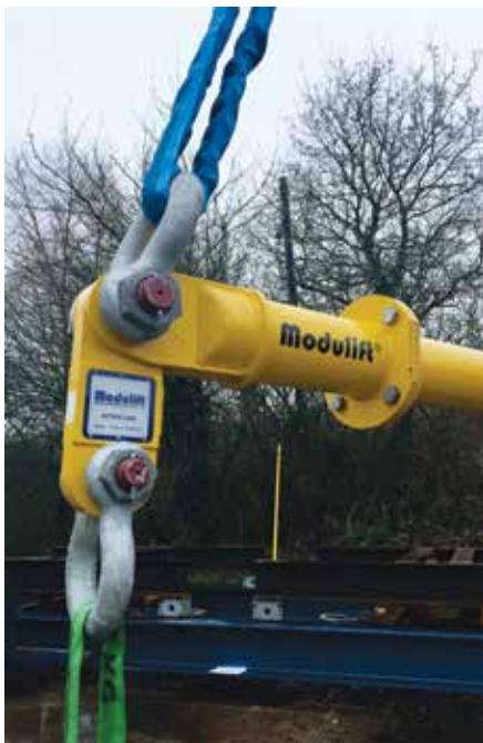
The new drop links are designed to fit standard end units, as well as the standard top and bottom shackles specified for the spreader.
